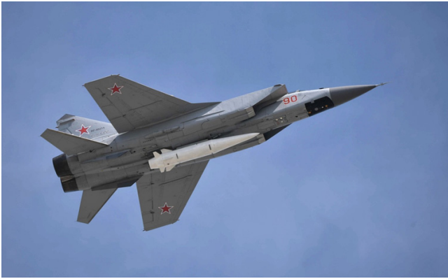
The Kh-47M2 Kinzhal (“dagger”) is a Russian hypersonic, nuclear-capable air-launched ballistic missile (ALBM). Seen here carried by MIG-31K interceptor fighter during the 2018 Moscow Victory Day Parade. Author: kremlin.ru, CC BY 4.0
