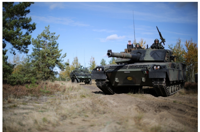
Italian Army - An Ariete main battle tank from the 4th Tank Regiment and a Canadian Army LAV III vehicle during exercise "Silver Arrow" in Latvia in September 2019. Author: Italian Army
