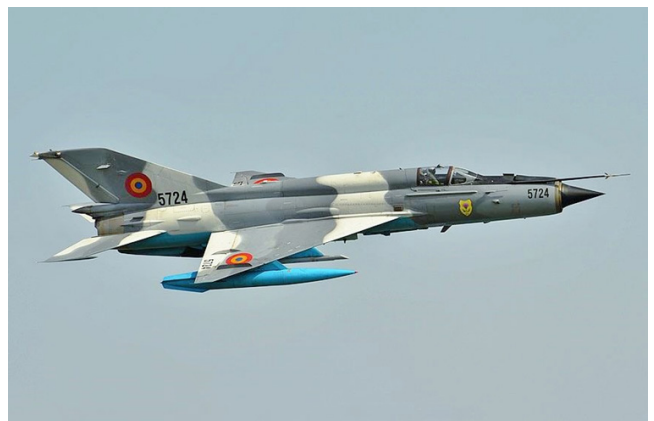
Romanian Air Force MiG-21 LanceR C in flight. LanceR variant planes were upgraded by Israeli firm Elbit Systems to modernise the old Soviet airframe and to make its equipment more compatible with NATO standards (the old SRZO-2 IFF transponder was replaced with IFF Plessey that is compatible with NATO IFF Mk. 10 transponder, according to STANAG 41-93. Author: Cristian Ghe, CC BY 2.0
